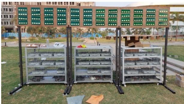
Outdoor testing of extreme massive MIMO
