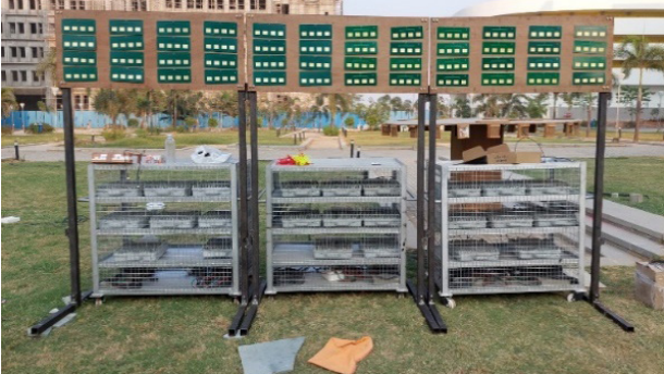
Outdoor testing of extreme massive MIMO
